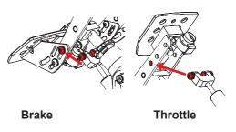
Turn the damper nut onto the damper towards the pedal lever. Stop when the damper bottom link side holes correspond with the damper nut side holes. Fix the damper nut onto the damper bottom link by tightening the two screws S3DK with Allen Key 2,5 mm.
