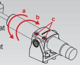
Now you can check the damper effect by pressing the pedal with attached and fixed ClubSport Pedals V3 Damper Kit. At the same time you can change the damper adjustment by turning the knurled plate at the back end of the damper, see picture below:
