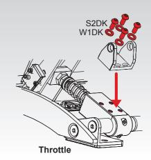
Attach the damper to the pedal lever at the marked holes and fix it by tightening the two screws S1DK to the throttle or the two screws already used to assemble the pedal extension on the brake by using Allen Key 4 mm. On the brake use the upper holes at pedal arm (where the pedal extension is also assembled), and on throttle use the lower holes at pedal arm:
