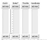
Above every indicator bar there are buttons labeled 'set max', and below every indicator bar there are buttons labeled 'set min'. These buttons are only available when checkbox 'Enable auto calibration mode' was deactivated by user before to enter manual calibration mode.
