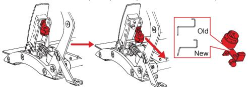
Attach the rumble motor upside down with the new rumble motor bracket at throttle pedal:
