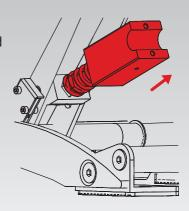
Attach the new spring with corresponding spring guides onto the pedal rod.
