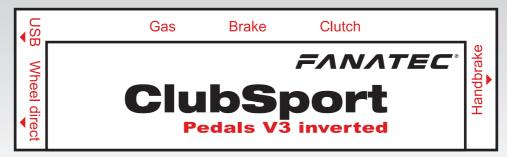
IMPORTANT: Connect the ClubSport Pedals either by USB cable OR by RJ12 cable to a wheel (base). Never connect both ways in parallel to avoid hardware damage!
