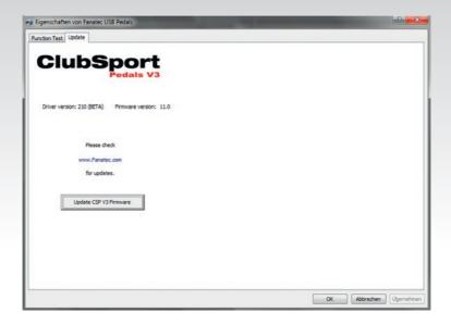
This page gives you detailed information about the currently installed PC driver version and the currently installed ClubSport Pedals V3i firmware version. There is also the button 'Update CSP V3 Firmware', see chapter 'Firmware update procedure' of this manual for more detailed information about the firmware update process itself.
