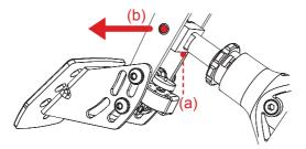
Disconnect the loadcell cable from 'Brake' port at the mainboard and take it out of the cable clips. Then turn the brake assembly downwards out from the brake pedal lever:
